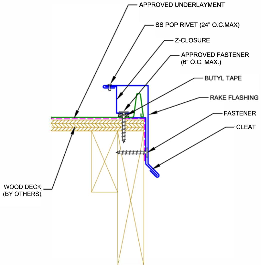
**NOTE:** 4" MIN. LAP ON DRIP EDGE WITH APPROVED SEALANT IN LAPS.
