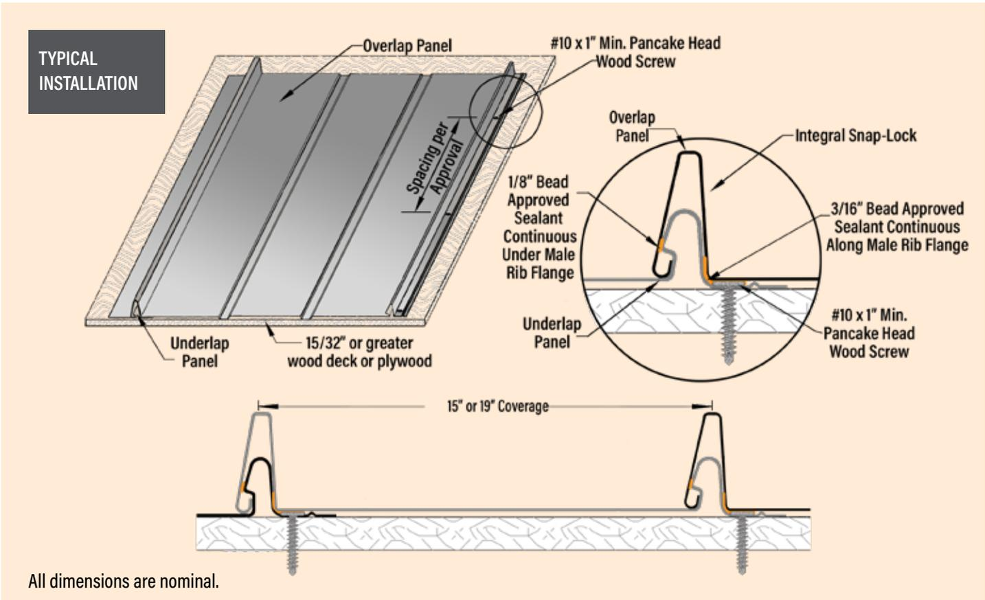
**!** Actual fastener pattern may vary from the pattern shown based on the specific roof plan, metal type and strength, local building codes and product approvals.
