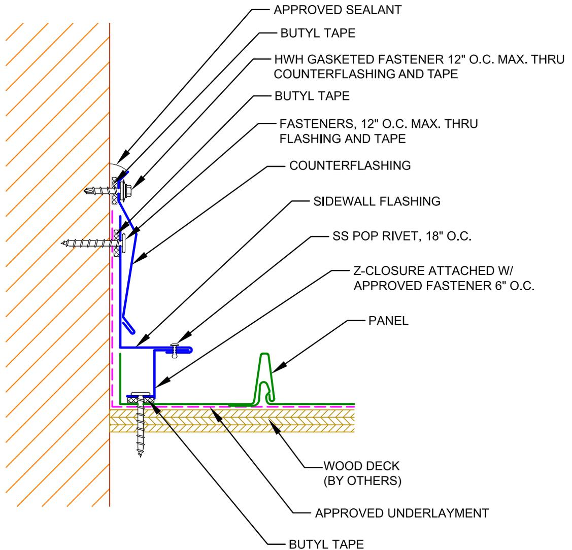
NOTE: 6" MIN. LAP ON SIDEWALL FLASHING WITH APPROVED SEALANT IN LAPS.
