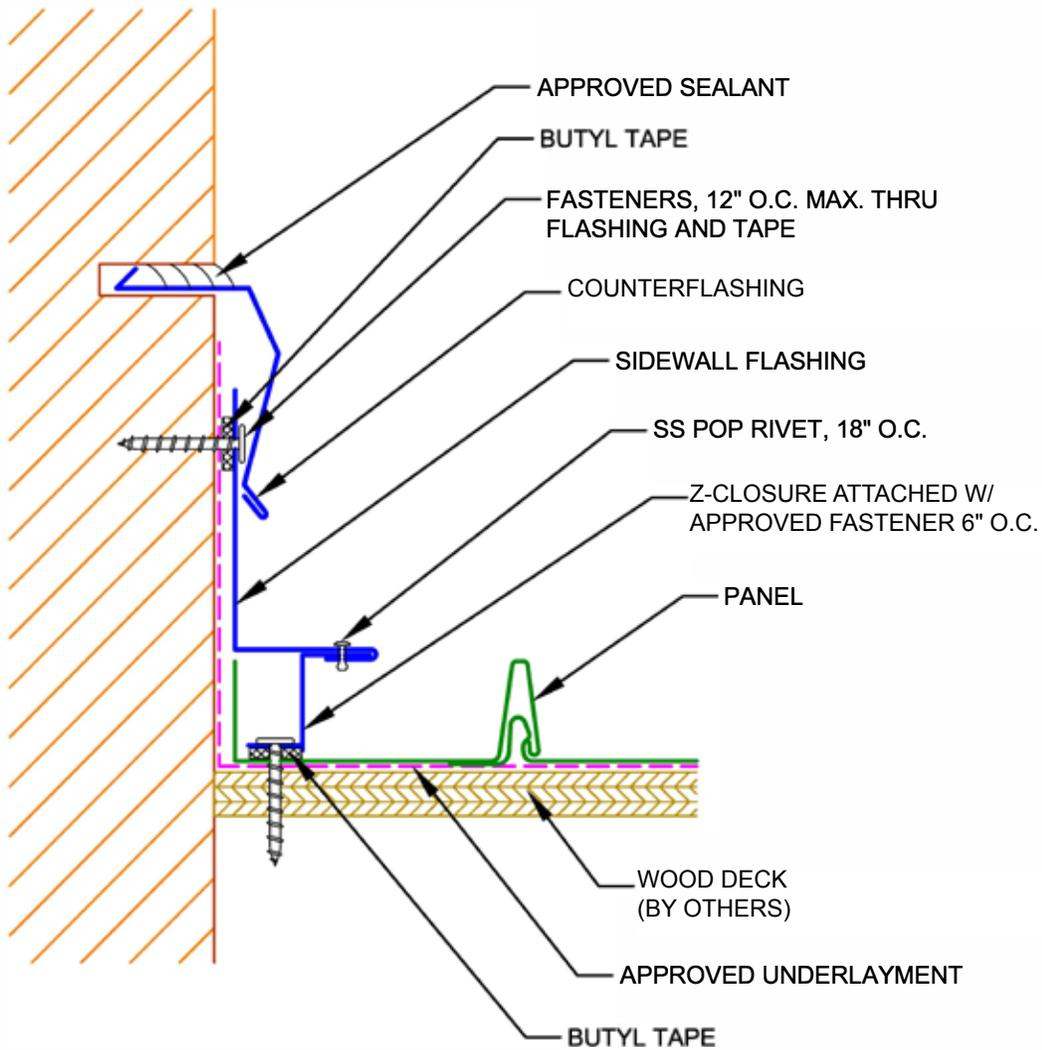
**NOTE:** 6" MIN. LAP ON SIDEWALL FLASHING WITH APPROVED SEALANT IN LAPS.
