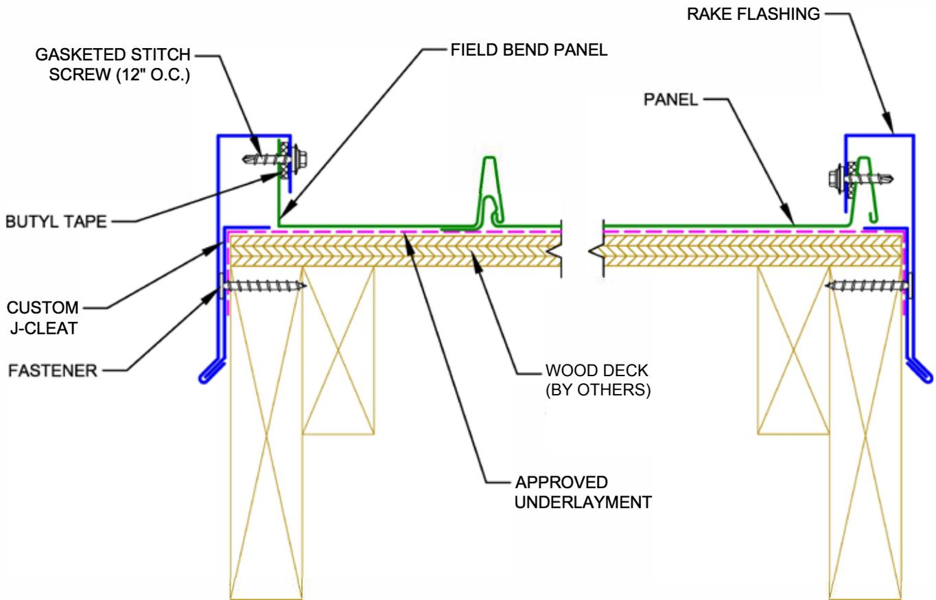
**NOTE:** 4" MIN. LAP ON RAKE DRIP EDGE WITH APPROVED SEALANT IN LAPS.
