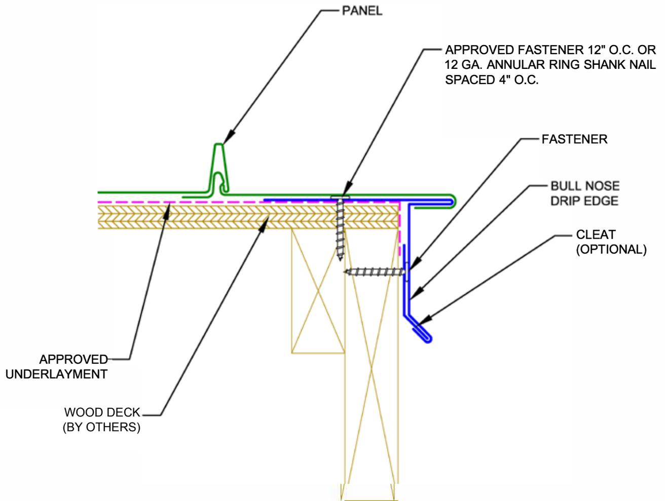
**NOTE:** 4" MIN. LAP ON RAKE DRIP EDGE WITH APPROVED SEALANT IN LAPS.
