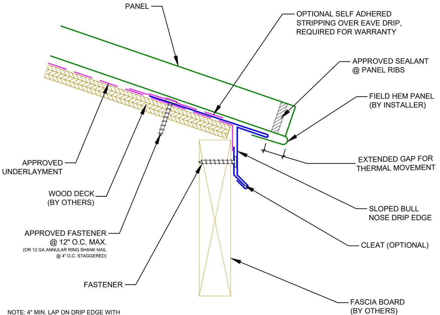
NOTE: 4" MIN. LAP ON DRIP EDGE WITH APPROVED SEALANT IN LAPS.
