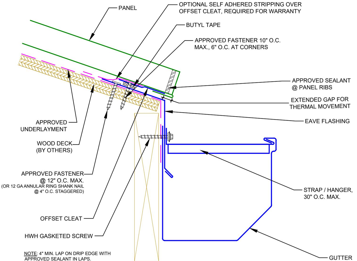
NOTE: 4" MIN. LAP ON DRIP EDGE WITH APPROVED SEALANT IN LAPS.
