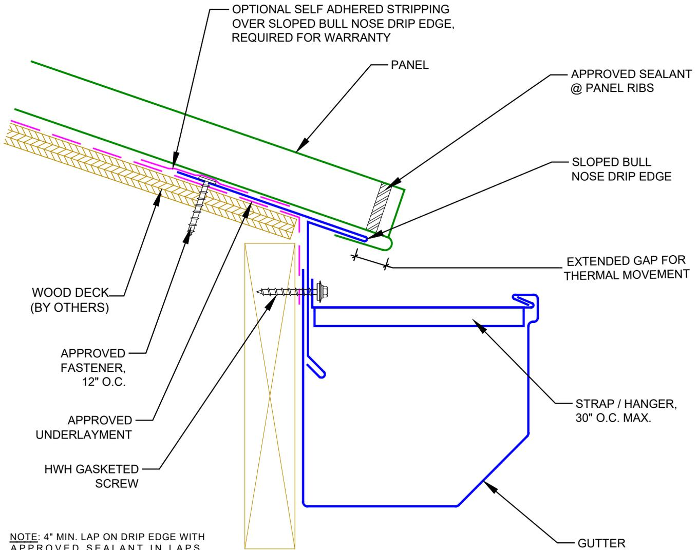
**NOTE:** 4" MIN. LAP ON DRIP EDGE WITH APPROVED SEALANT IN LAPS.
