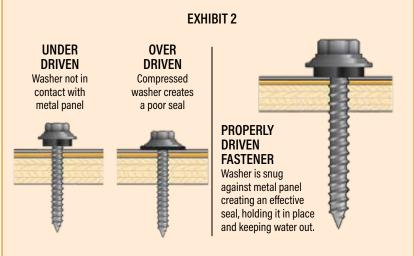
a different size replacement fastener as needed. If distortion or damage is too severe, replacement of the metal panel may be necessary.
