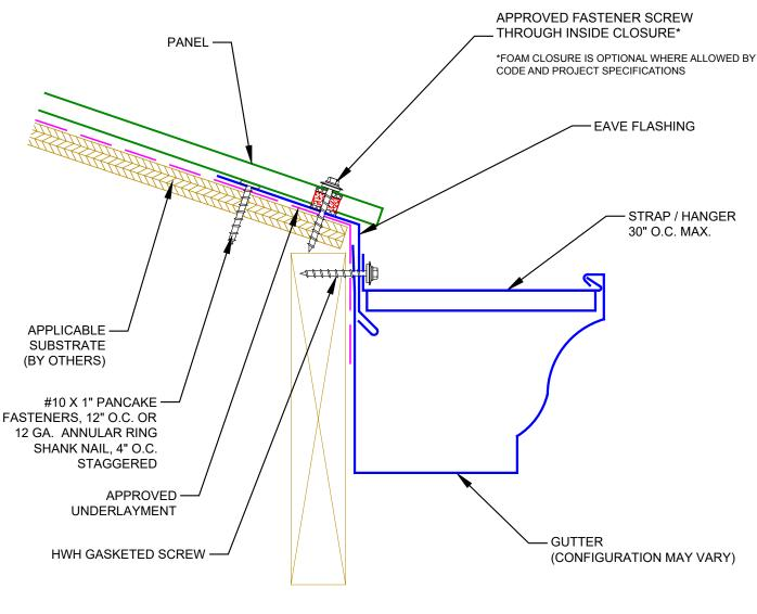
NOTE: 4" MIN. LAP ON DRIP EDGE WITH APPROVED SEALANT IN LAPS.
