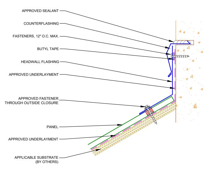
NOTE: 6" MIN. LAP ON HEADWALL FLASHING WITH APPROVED SEALANT IN LAPS.
