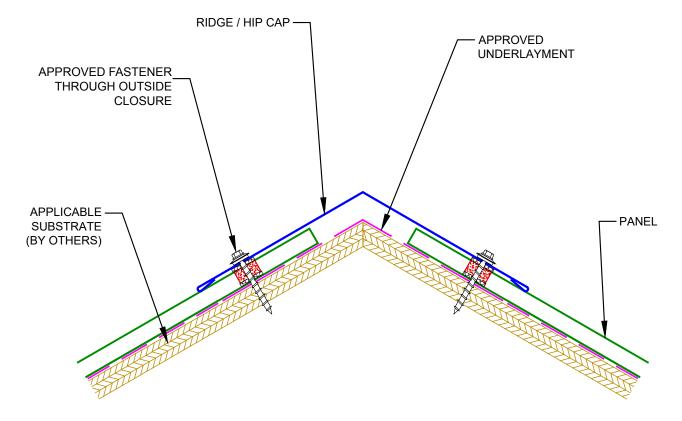
NOTE: UNIVERSAL CLOSURE USED AT HIPS <u>OPTION:</u> 6" WIDE PEEL AND SEAL TAPE IS AVAILABLE TO SEAL OVER PANELS PRIOR TO INSTALLING RIDGE CAP
