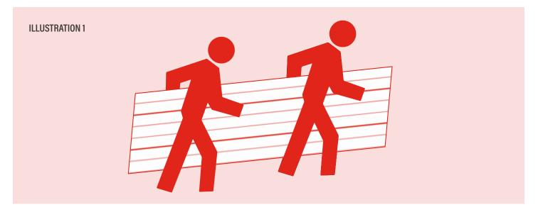
Once a bundle is opened, individual panels must be handled with care to prevent panel buckling or finish damage. Never slide a panel over another panel when removing it from the bundle. A panel should be lifted up from the bundle in order to minimize the possibility of damaging the finish.
