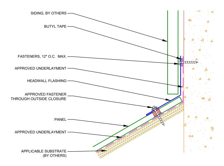
$\underline{\text{NOTE}}$ : 6" MIN. LAP ON HEADWALL FLASHING WITH APPROVED SEALANT IN LAPS.
