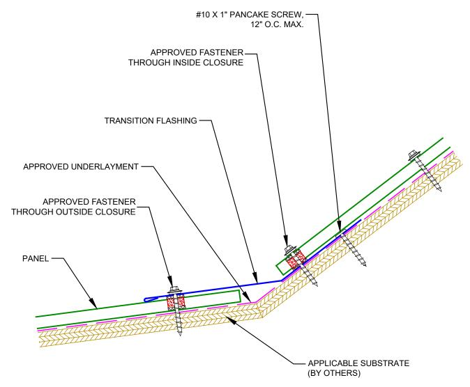
NOTE: 6" MIN. LAP ON TRANSITION FLASHING WITH APPROVED SEALANT IN LAPS.
