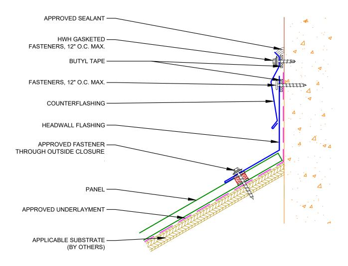
$\underline{\text{NOTE}}$ : 6" MIN. LAP ON HEADWALL FLASHING WITH APPROVED SEALANT IN LAPS.
