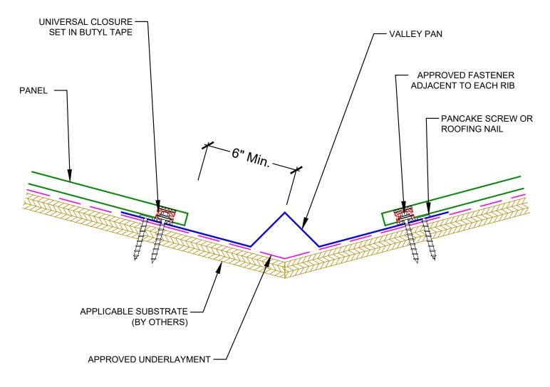
NOTE: FLASHING LAPS IN VALLEY ARE 6" MIN. USE TWO ROWS OF APPROVED TUBE SEALANT IN ALL LAPS.
