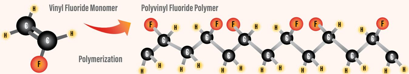
The precursor of polyvinyl fluoride (PVF) is vinyl fluoride (VF), an organic compound of carbon, fluorine, and hydrogen.
